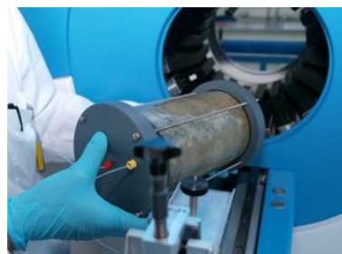
Analysis of tracer flow with GeopET (HDZR)
