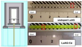
**Fig. 1.** Schematic representation of the hot zone for  $\mu$ -PD crystal growth (left; white: Ir, gray: ceramics, blue: fused silica) and grown Lu<sub>3</sub>Al<sub>5</sub>O<sub>12</sub> crystals (right).
