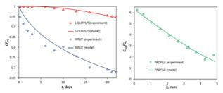
**Fig. 2.** Results of Sr (labelled by <sup>85</sup>Sr) through-diffusion experiment, which lasted 22 days, in portlandite equilibrated water and its optimal fit.
