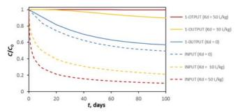
**Fig. 1.** Modelled time dependences of concentrations in input and output containers (60 mL); parameters of the layer: diameter 50 mm, width 10 mm, porosity 0.5,  $D_p = 1 \cdot 10^{-10} \text{ m}^2 \text{s}^{-1}$ ) for three values of distribution coefficient  $K_d$ .
