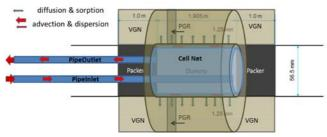
**Fig. 1.** The graphical representation of the conceptual model. Inlet and outlet PEEK tubing were modelled by two Pipe pathways. An annular slot and rock matrix were modelled by Cell pathway network of a cylindrical geometry.
