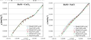
Fig. 2. Sorption isotherms of Cs on bentonite BaM (points) in CaCl<sub>2</sub> background electrolyte (left) and NaCl background electrolyte (right) and prediction of ion exchange/surface complexation model (lines) for three solid-to-liquid ratios.
