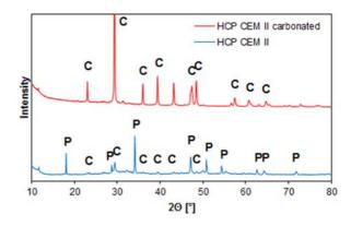
**Fig. 1.** XRD analysis of HCP CEM II prior and after carbonation. C – Calcite, P – Portlandite.
