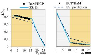
**Fig. 2.** Experimental, GoldSim (GS) fitted and predicted (from the individual system) HTO concentration profiles in the coupled system.
