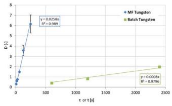
**Fig. 1.** Non equilibrium D(W) dependency on contact time for the 0.5M Cy600/0.5M HNO<sub>3</sub> system. Slug-flow microfluidics (blue) vs. Grant Bio PTR30 rotator-mixer (green).
