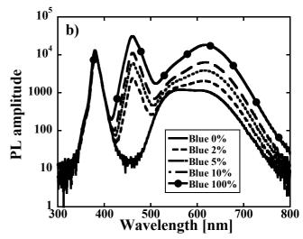
**Fig. 1.** Overall emission spectra of the circadian light source with a K<sub>0.8</sub>Na<sub>0.2</sub>LuS<sub>2</sub>:Eu<sup>2+</sup> sample (fraction of big crystals), fixed nearUV LED power (10 %) and varying blue LED power [2].
