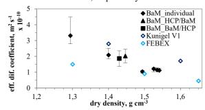
**Fig. 1.** HTO effective diffusion coefficients on compacted BaM (individual and coupled systems). Comparison with Kunigel V1 [4] and FEBEX [5].
