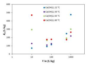
**Fig. 1.** Dependence of determined  $K_d$  values describing  $^{223}$ Ra uptake on hydrated cement paste in the Portlandite water Ca(OH)<sub>2</sub> on the phase ratio V/m at different temperatures.
