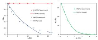
**Fig. 3.** Results of <sup>223</sup>Ra through-diffusion experiment of, which lasted 22 days, in portlandite equilibrated water and its optimal fit.
